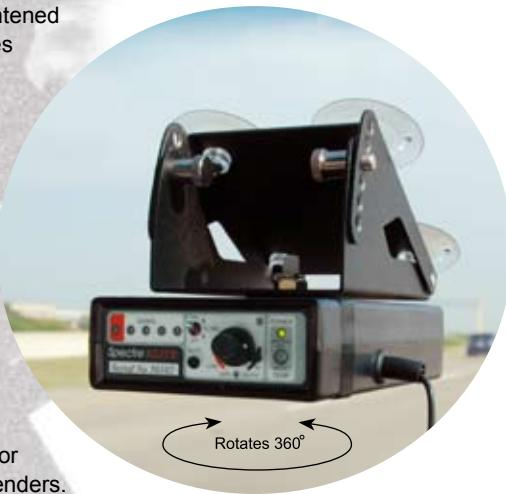
The Spectre ELITE is about the size of today's radar detectors and mounts to the windshield of the patrol vehicle. It can be rotated 360 degrees to detect detectors at all angles relative to the vehicle.
